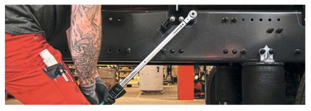
With modern worker guidance, tools are available to prevent errors in screw connections from the outset. (Image: Stahlwille)
